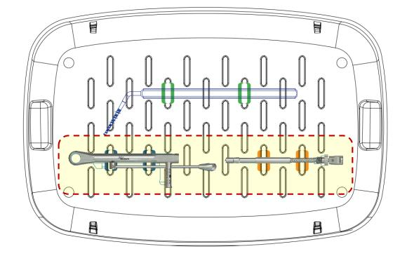
⇒ Torque Ratchet must be separated and stored after cleaning and sterilization.
